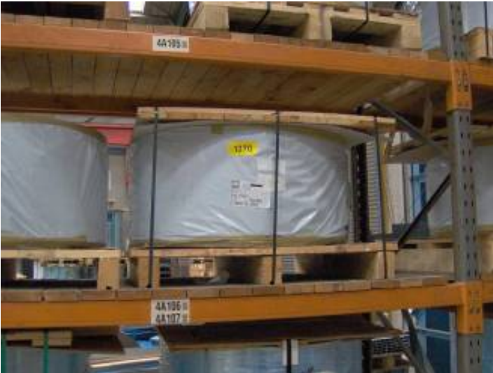
'Eye to Sky' coil packed on a pallet with a lid and banded securely.
